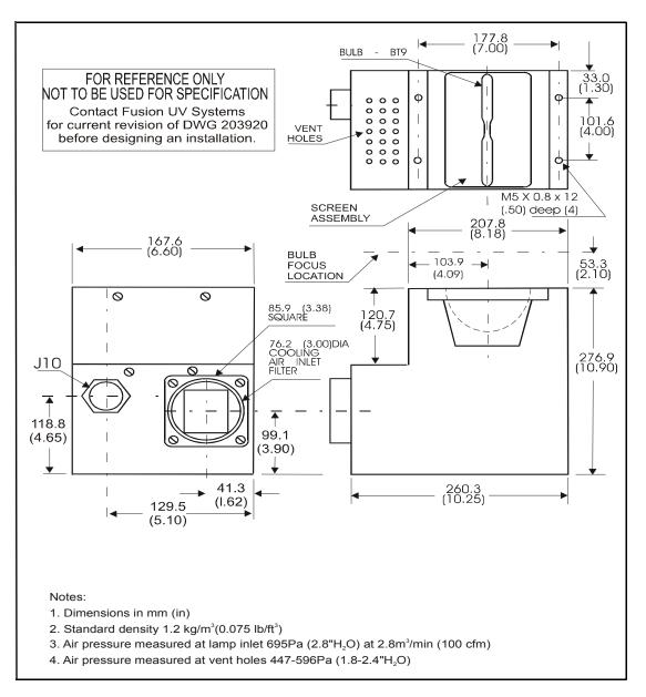
Figure 52. I300M Irradiator Dimensions
